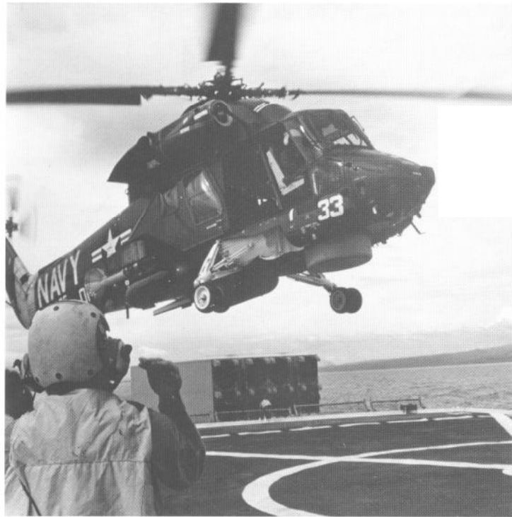
An LSE (landing signal enlisted) directs a Kaman SH-2F Seasprite to a safe landing on the deck of the frigate Lang (FF-1060). Such helicopters are used to extend the range of surface ships in antisubmarine warfare. K 109843
