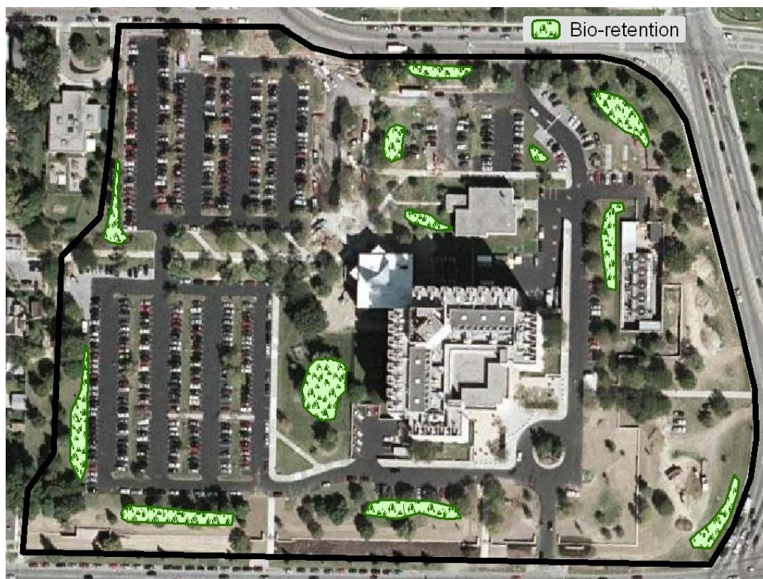
Figure 14. Actual Site and Onsite Control Measures (Cincinnati, OH)
