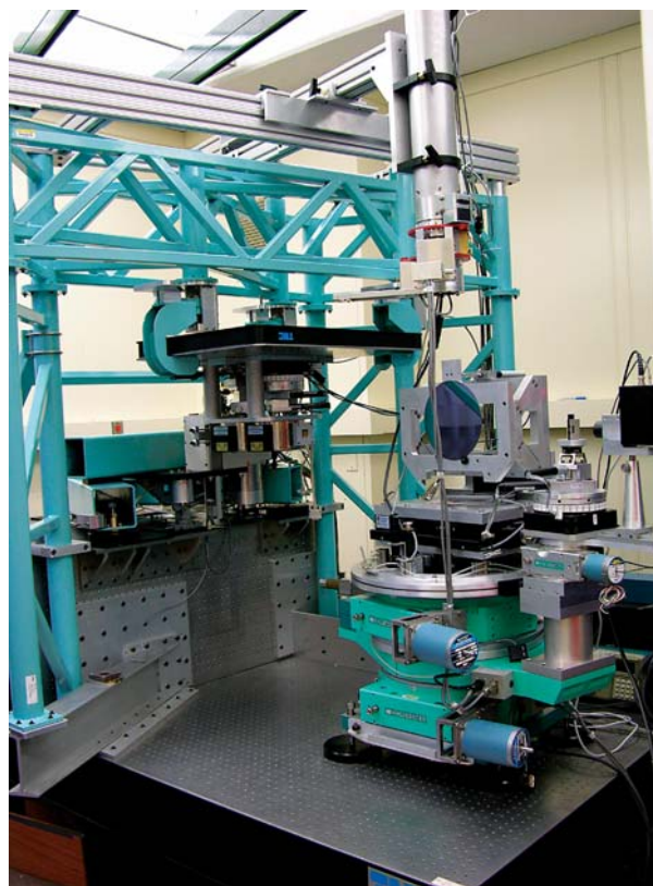
Figure 3: The Ceramics Division Parallel Beam Diffractometer in the AML.
