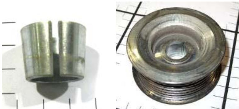
Figure 2-22: Motor Generator Pulley
