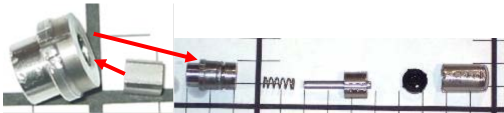
Figure 3-20: (Left) Magnetic Reaction Mass and Rod, (Right) Cylinder, and Reaction Mass Assembly
