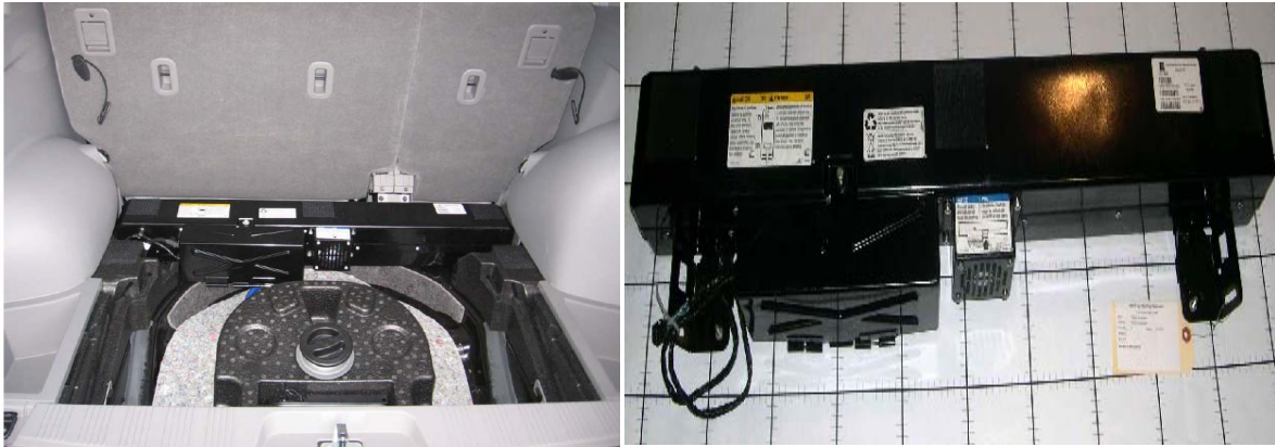
Figure 2-38: Saturn Vue Green Line 36V Battery Pack Installed in Vehicle (LHS) and Removed from Vehicle (RHS)
