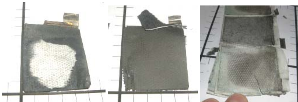
Figure 2-45: Positive Anode, Negative Anode and Separator paper
