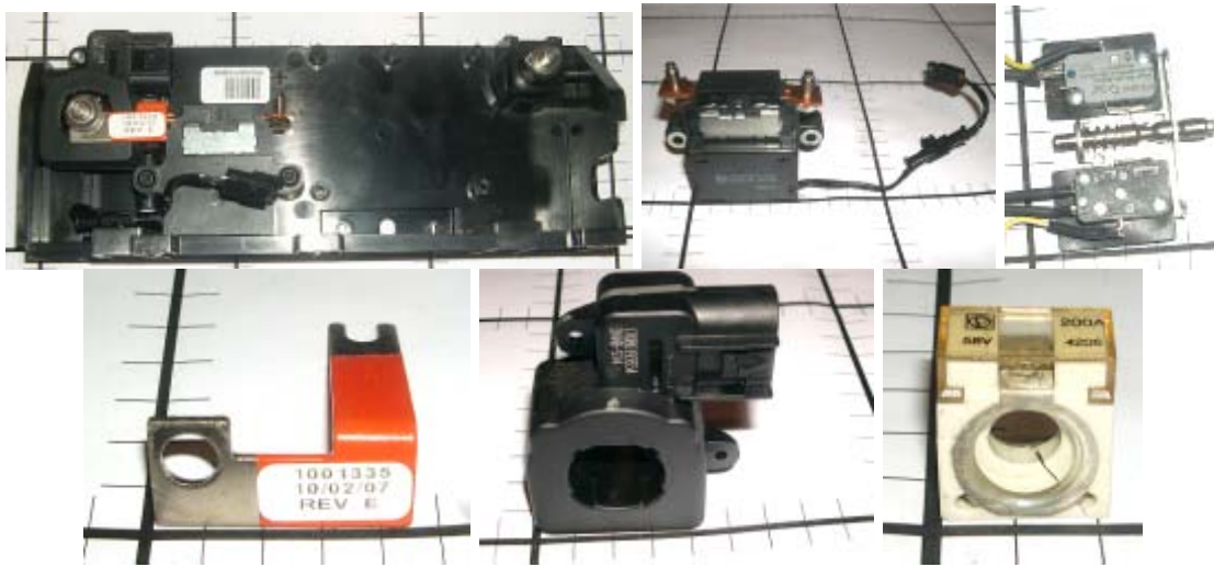
Figure 2-49: (clockwise from top left) Disconnect Box, Disconnect Relay, Switch, Bus bar, Current Sensor, and Fuse
