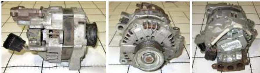
Figure 2-21: Motor Generator Assembly Assorted Views
