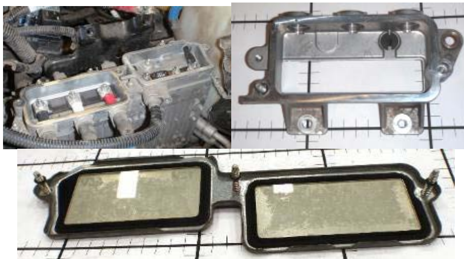
Figure 2-55: SGCM Cable Interfaces
