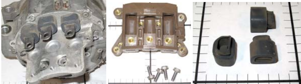
Figure 2-25: Cable Interface Block
