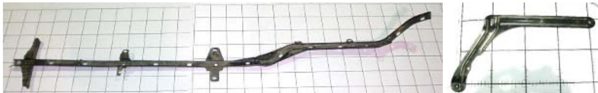
Figure 2-52: Cable Protective Covers
