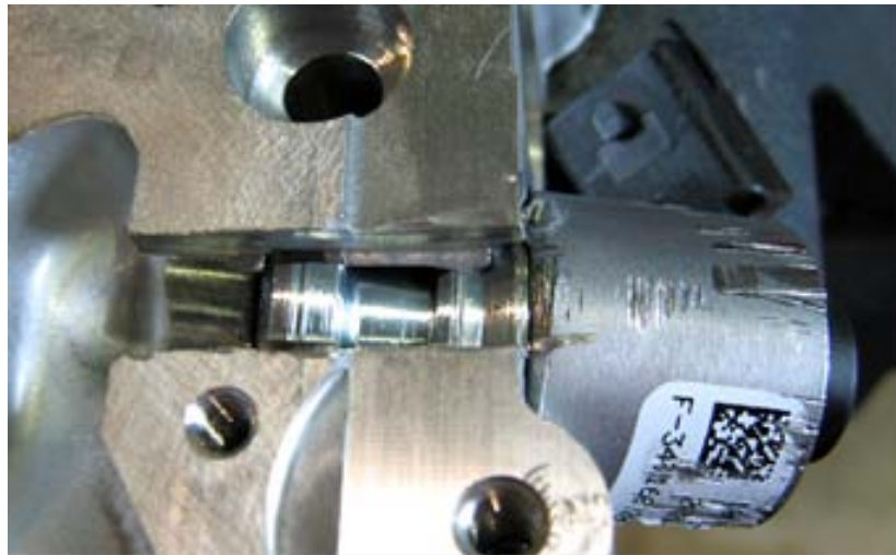
Figure 3-14: Solenoid pressed into manifold bore
