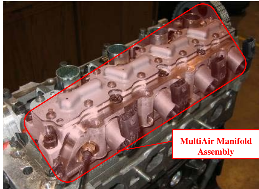
Figure 3-2: MultiAir Manifold Assembly Installed on the Fiat 1.4L, I4, ICE
