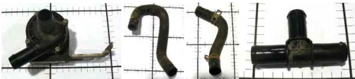
Figure 2-4: Heater Core Coolant Electric Circulation Pump
