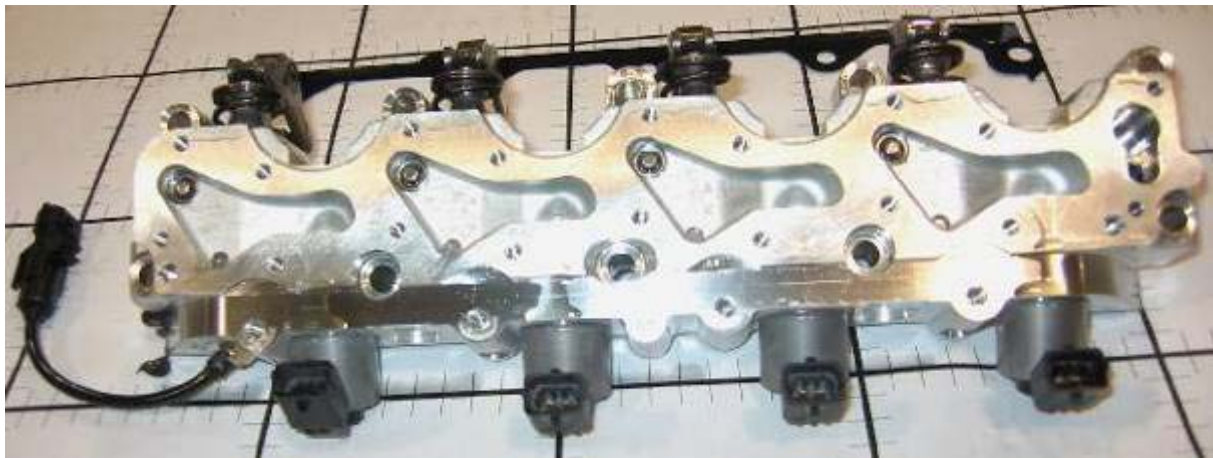
Figure 3-3: MultiAir System Forged Aluminum Manifold
