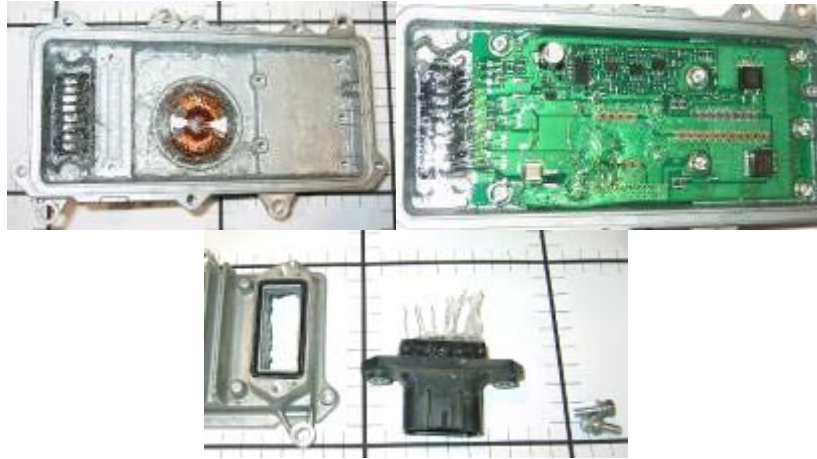
Figure 2-58 : 8-Pin Module Electrical Components
