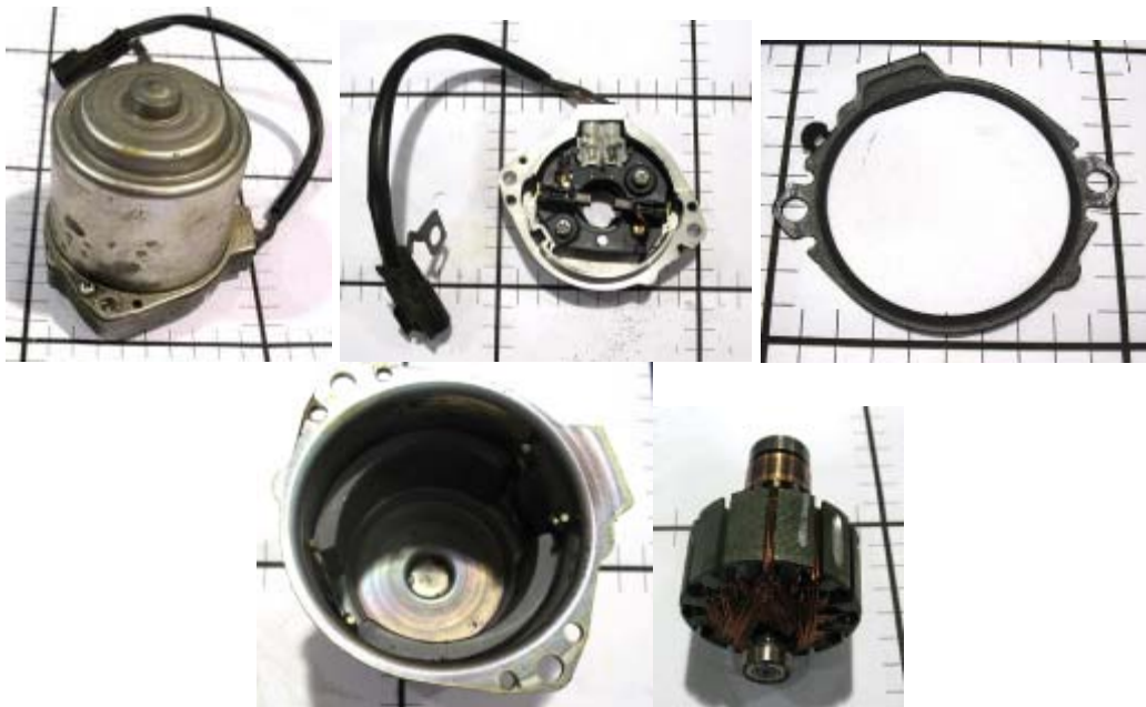
Figure 2-10: Oil Pump Electric Drive Motor
