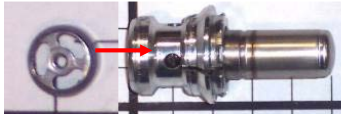
Figure 3-19: Solenoid Oil Outlet Port (Pressed into the Valve Housing Oil Dump Outlet)
