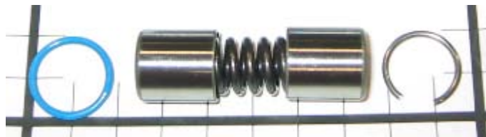
Figure 3-25: Oil Reservoir Pressure Relief Valve
