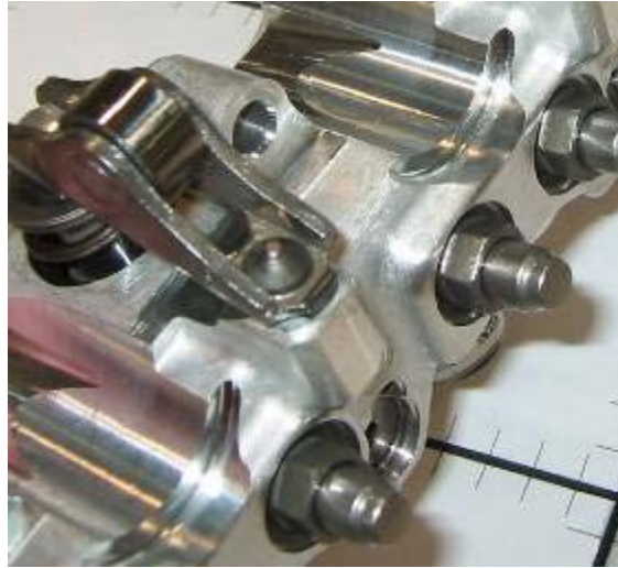
Figure 3-10: Hydraulic Brake and Lash Adjusters (HBLA) in Hydraulic Manifold
