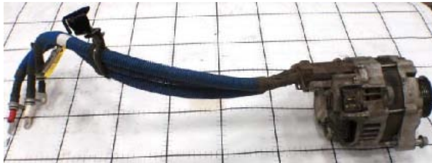
Figure 2-20: Motor Generator Removed
