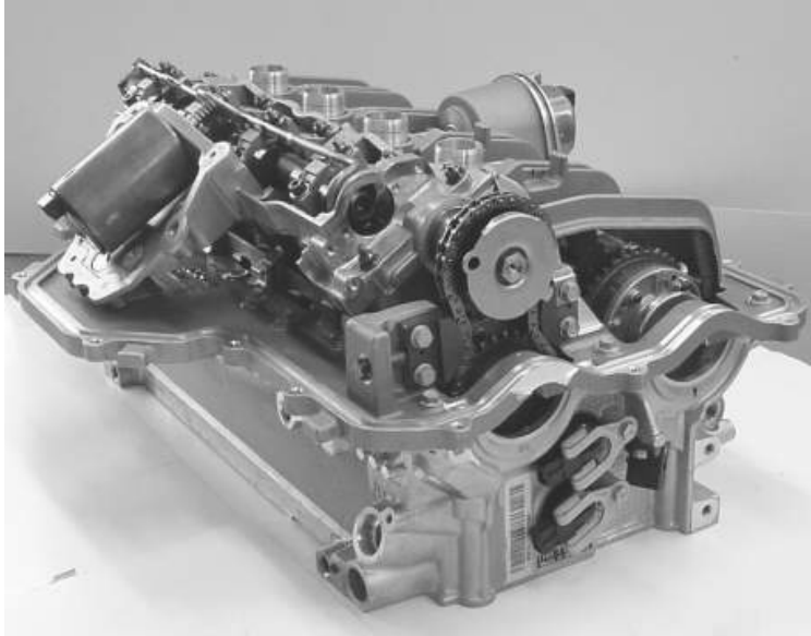
Figure 5-16: Ricardo TMVL (Twin Mechanical Variable Lift) HCCI research cylinder head assembly
