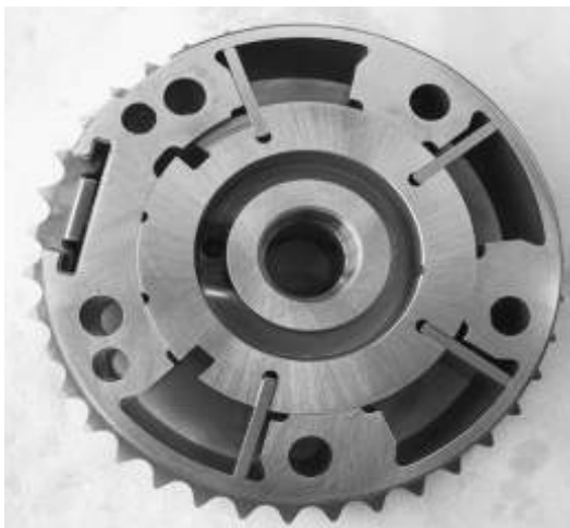
Figure 5-1: Hydraulic vane-type cam phaser
