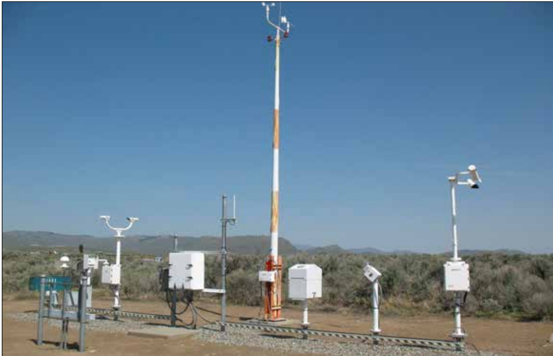
Figure 6-33. ASOS Weather Sensors Suite
