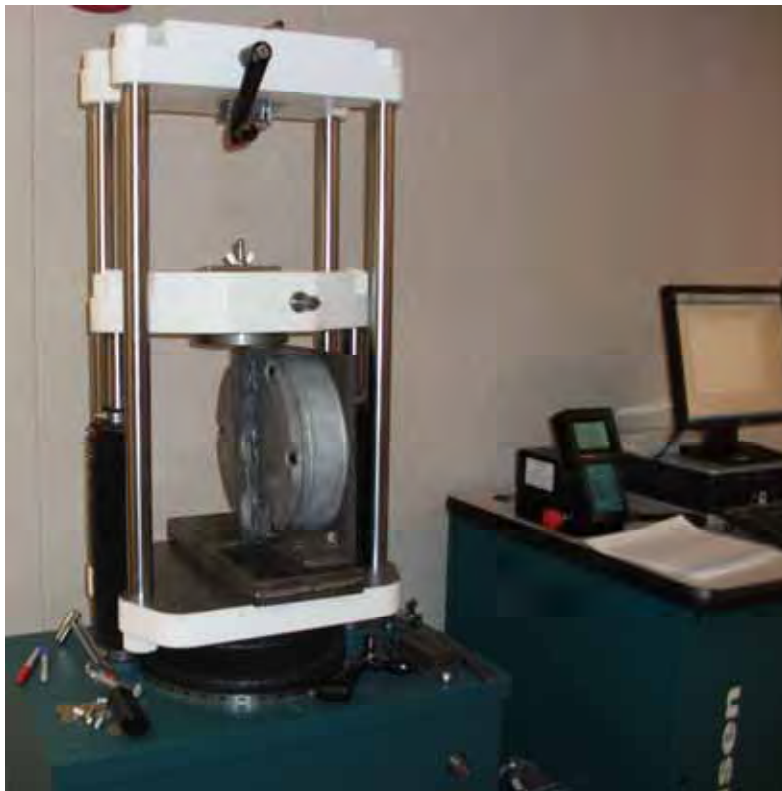
Figure 14. Tinius Olsen Computerized Hydraulic Tester With Test Fixture Mounted
