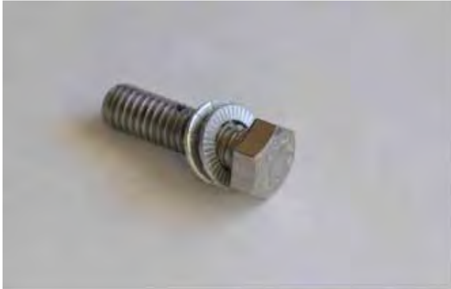
Figure 3. Two Part Locking Washers Installed on a 3/8-inch Tap Bolt
