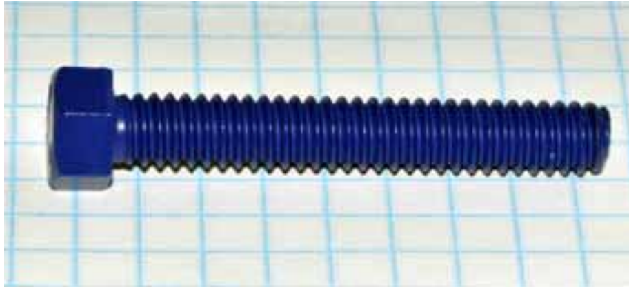
Figure 6. An Example of a Ceramic-Metallic/Fluoropolymer Coated 3/8-16 X 2 Inch Bolt
