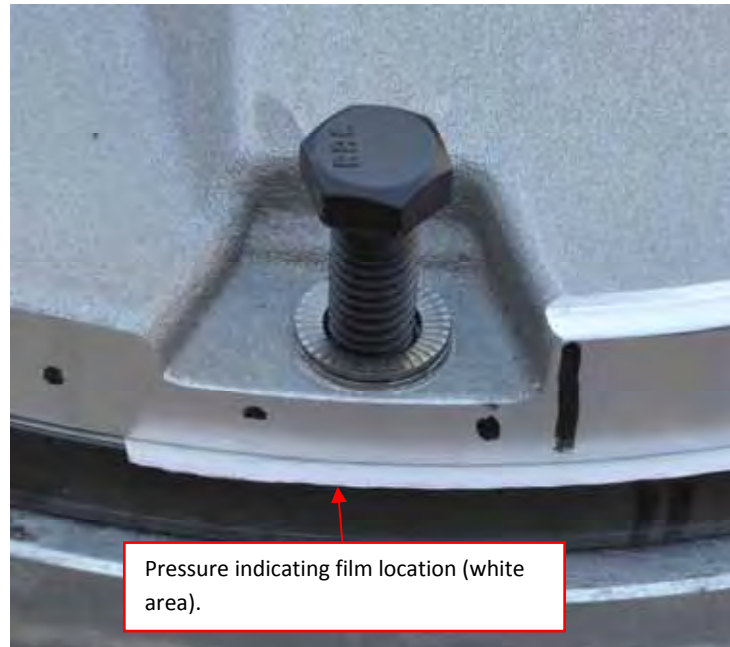
Figure 8. Coated Bolt and Two Part Washers
