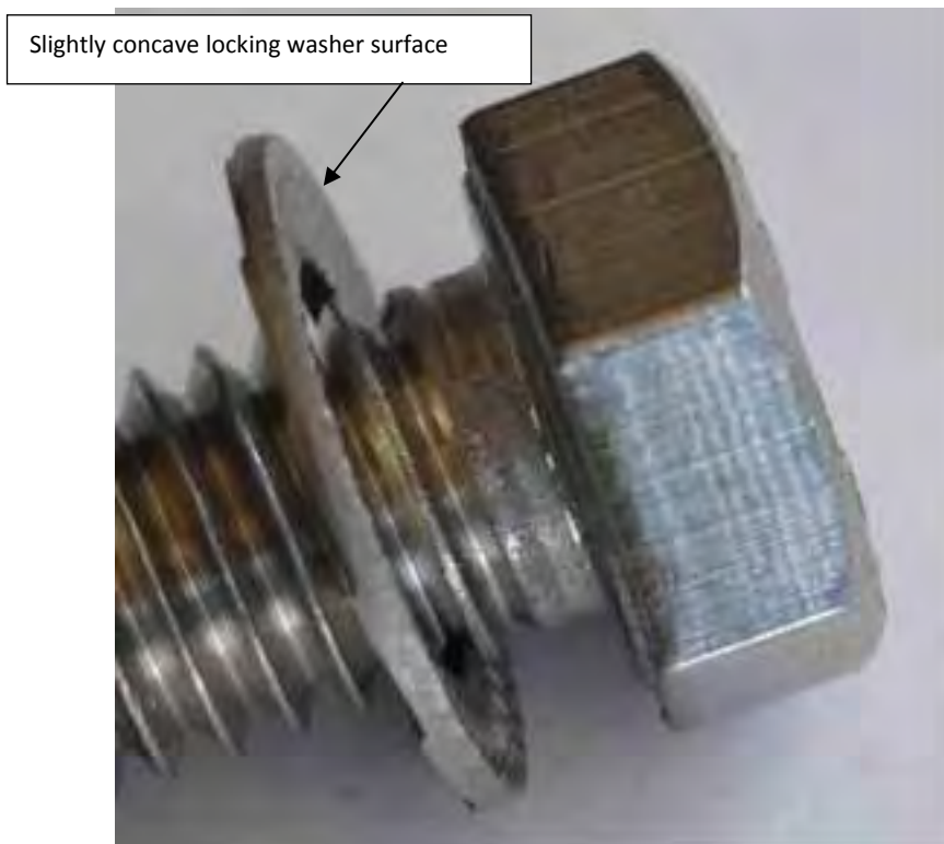
Figure 4. Bolt With a Slightly Concave Upper Locking Washer (bolt tightened to 15 ft. lbs.)
