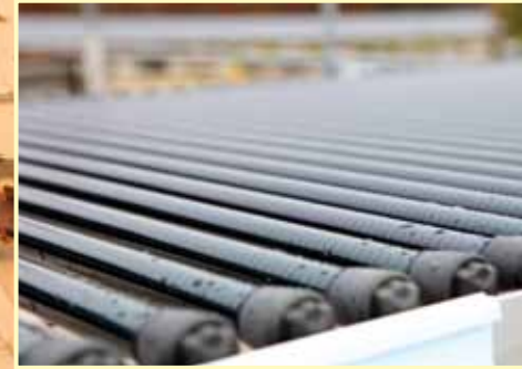
The Large-Scale Climate Simulator can enclose roof or wall sections within a highly customizable micro-climate.
