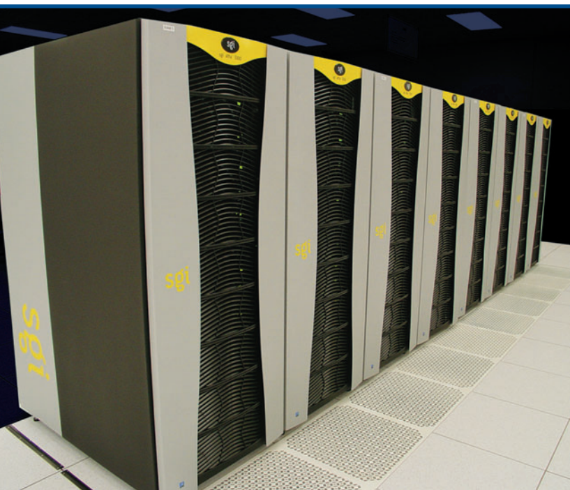
The SGI Altix supercomputer at CCS has a huge memory. It can hold up to 2 trillion bytes of data.
