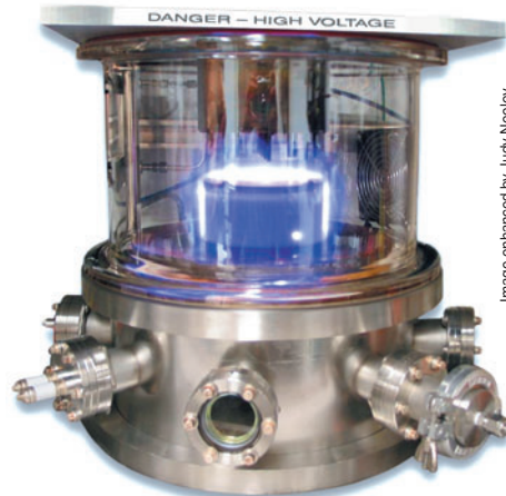
This plasma-enhanced chemical vapor deposition device at ORNL is used to grow patterned carpets of carbon nanofibers on silicon substrates for possible electronic applications.
