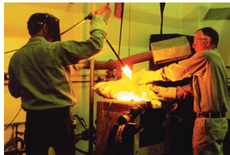
ORNL's Ed Hatfield and Joseph Vought prepare to carry out a lost-foam metals-casting operation.
