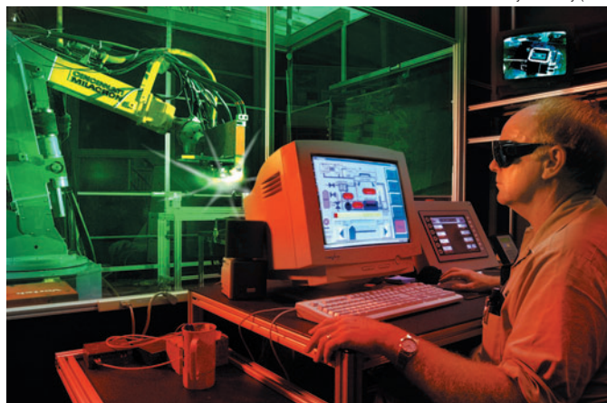
ORNL's David Harper performs materials processing using the robotically controlled plasma arc lamp.
