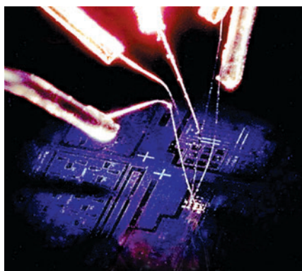
First transistor fabricated at ORNL, described in an October 2001 issue of Science magazine. The gate oxide is strontium titanate, which performs better than silicon dioxide materials, now used in metal oxide field effect transistors.
