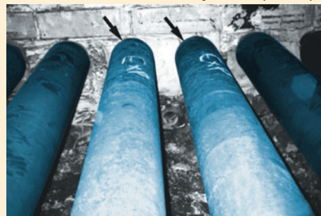
Conventional steel rolls at Bethlehem Steel (left and right) form blisters that cause undesirable surface blemishes in steel plates, the product of the steel mill. Rolls made of ORNL-developed nickel aluminide (center, with arrows) show no signs of blistering.
