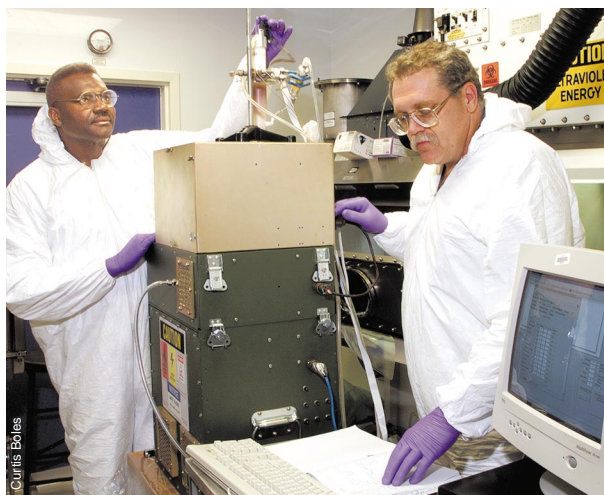
Roosevelt Meriweather and Rob Smith check the operation of the chemical biological mass spectrometer developed partly by ORNL researchers for use in helping U.S. Army soldiers detect the presence of biological and chemical warfare weapons.
