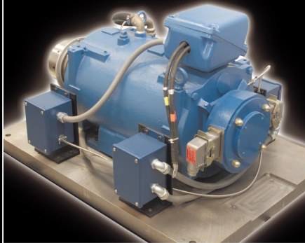
This diesel engine will be tested for speed and power on a dynamometer at NTRC. (See p. 5.)
