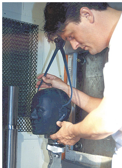
Tyler Kress measures the dimensions of a dummy head after subjecting it to airbag testing in a laboratory at Southern Impact Research Corporation.
