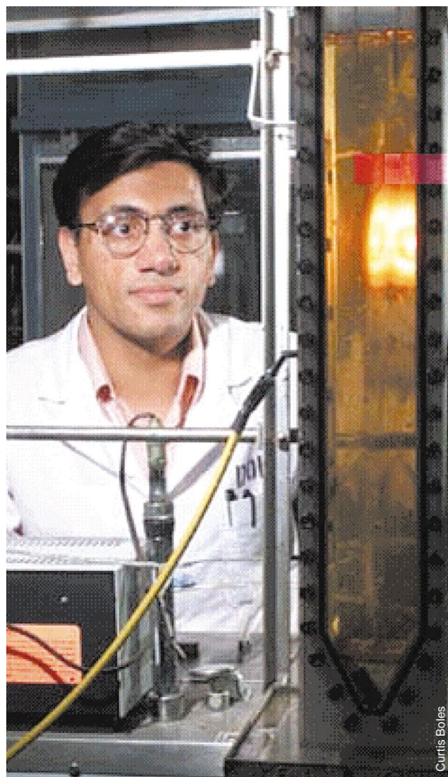
Abhijeet Borole checks the operation of a bioreactor that uses suspended bacteria to remove sulfur from petroleum feedstocks.
