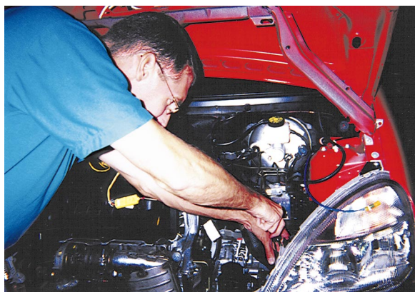
Brian West checks a Mercedes A170 diesel engine, which is being tested to determine the efficiency of its emissions control system in removing nitrogen oxides and particulate matter from its exhaust. The engine is run on an ORNL stationary engine dynamometer, which applies the same resistance to the engine as the road would if the engine were connected to wheels. Top photo enhanced by Gail Sweeden.
