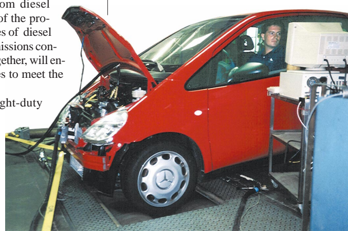
The effects of low-sulfur fuel on a diesel engine's emissions control system (top) were studied by ORNL researchers using this Mercedes diesel car on a University of Tennessee chassis dynamometer (bottom). ORNL's Scott Sluder is in the car.
