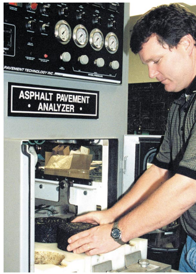
Mike Jackson evaluates the anticipated performance of pavement samples in this testing device. He hopes to identify longer-lasting pavement materials.
