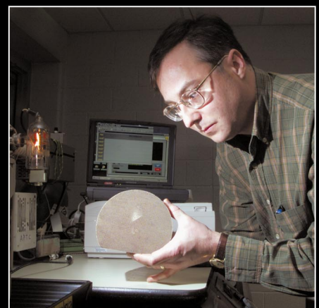
Bill Partridge prepares to use a mass spectrometer to analyze the effectiveness of diesel fuel hydrocarbons in regenerating a catalyst used to remove nitrogen oxides from engine emissions. (See p. 5.)
