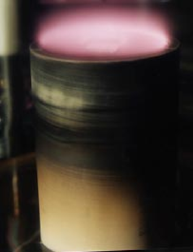
The pink glow enveloping the square sample results from plasma-induced chemical vapor deposition, which is used to grow carbon nanotubes. The sample has a layer of a metal catalyst, such as iron or nickel, to promote nanotube growth.
