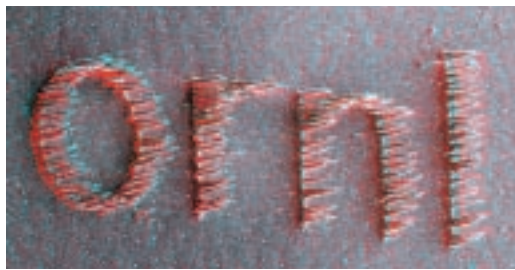
The Laboratory's initials have been constructed from carbon nanotubes using plasma-induced CVD on pre-deposited catalyst patterns. The letters are started by forming a pattern using electron beam lithography followed by electron-gun evaporation of the iron catalyst.
