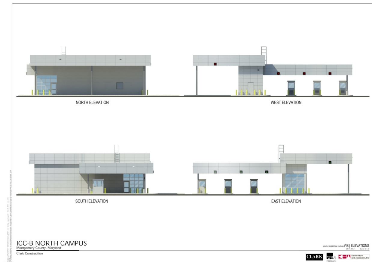
Figure 12: Elevations of the Vehicle Inspection Station.
