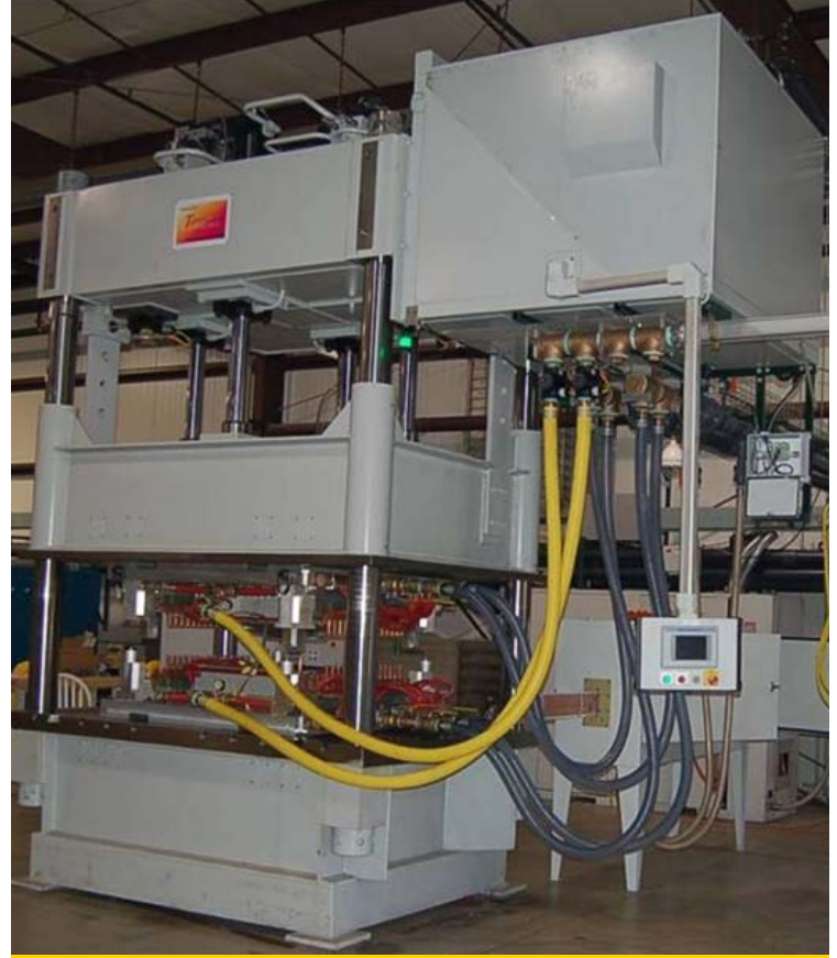
Induction molding press with seatback tool installed in the press at AjaxTOCCO, Madison Heights, MI.
