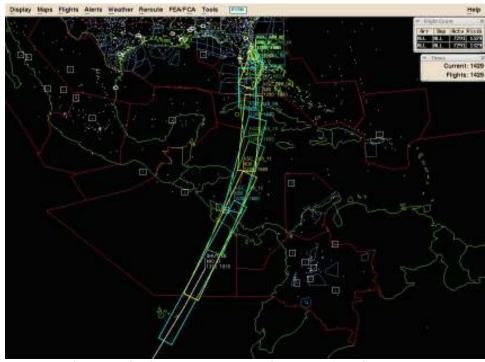
Figure 5. TSD Shuttle Reentry Debris Hazard Area Screenshot.
