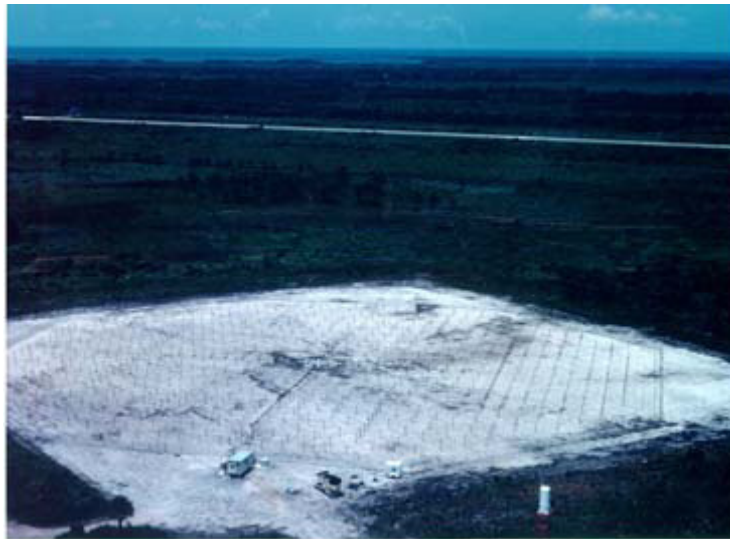
Figure 3-2. 50-MHz DRWP Antenna Field Located at KSC [Fig. 3, Decker and Leach, 2004. Image reprinted with permission of authors.]
