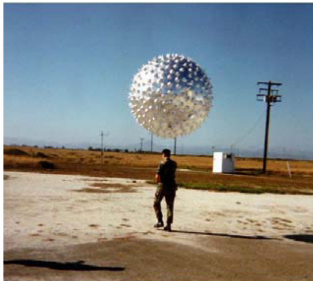
Figure 3-9. Jimsphere Balloon Used for High Resolution Wind Measurements [Fig. 1, Decker and Leach, 2004. Image reprinted with permission of authors.]
