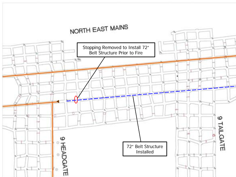
Figure 5. Critical ventilation control removed prior to fire.
