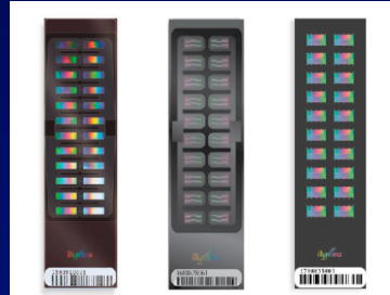
Infinium Assay BeadChips enable interrogation of ~317,000 to over one million SNPs and offer comprehensive coverage of CNV regions. Shown above, from left to right, are the Human100K-Duo, Human550K-Duo, and Human1M BeadChips.
