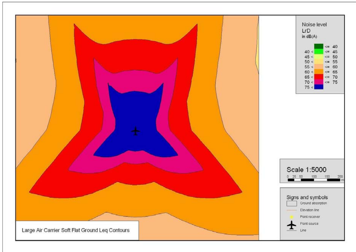
Figure 12 Large Air Carrier (Boeing 737-300) A-weighted Taxi Noise Emission Directivity
