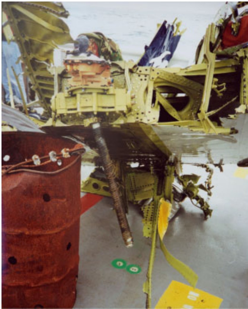
Figure 12a. The acme screw immediately after it was brought on board the recovery ship.
