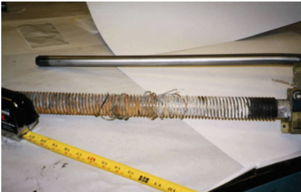
Figure 13. A photograph of the acme screw thread remnants wrapped around the screw, the red rust areas, and the white deposits.
