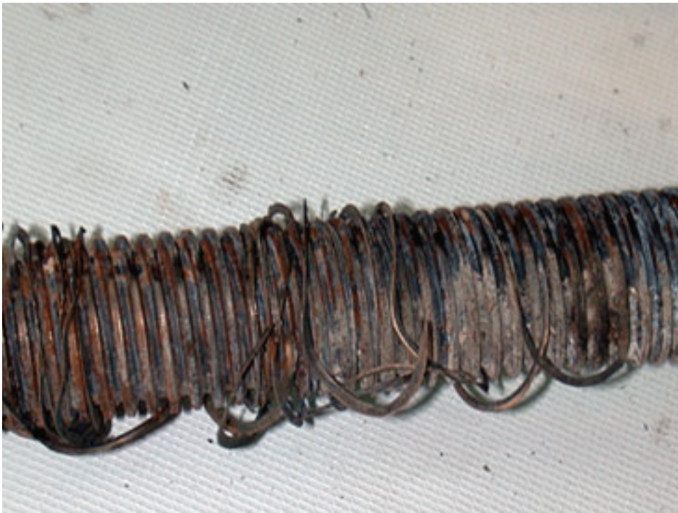
Figure 12c. The acme screw during initial inspection.
