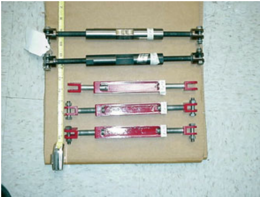
Figure 10. Two Alaska Airlines-fabricated restraining fixtures and three Boeing-manufactured fixtures.
