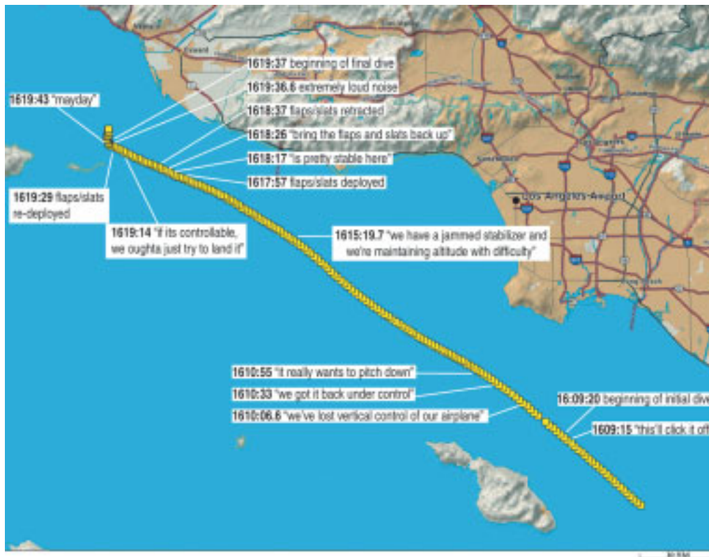
Figure 1. The accident airplane’s flightpath, starting about 1609 (about the time of the initial dive) and ending about 1620 (about the time of the second and final dive).
