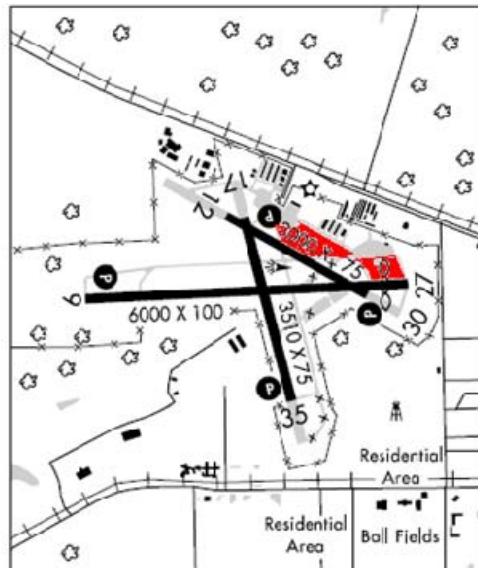
Figure 10. Palatka Municipal Airport, FL, A/FD
