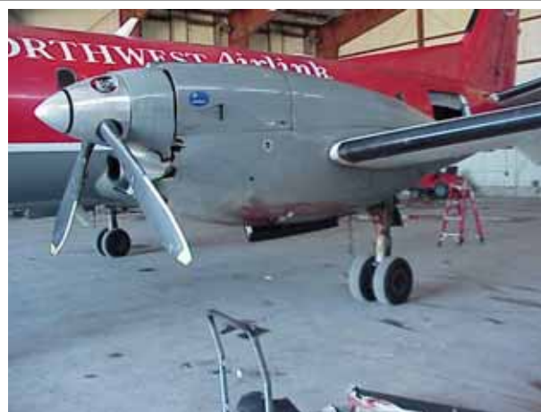
This Saab 340 hit a deer on landing at a Midwest USA airport in April 2000, ripping the engine from its mountings (photo courtesy Northwest Airlines).
