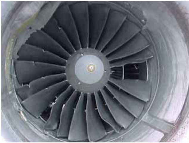
This picture shows a close-up of the #2 engine from the Fokker-100 that ingested Canada geese on 4 September 2004.
