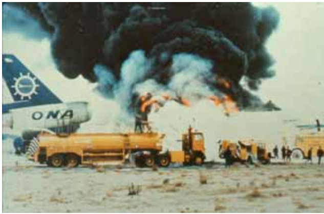
This DC-10 was destroyed by fire when several herring gulls were ingested into an engine during takeoff from JFK International Airport, November 1975 (see story on page 17; photo courtesy Port Authority New York and New Jersey).
