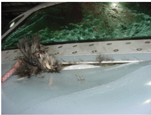
One of the two turkeys that penetrated a Canadair RJ 200 fuselage below the windshield; parts of the bird entered the cockpit.
