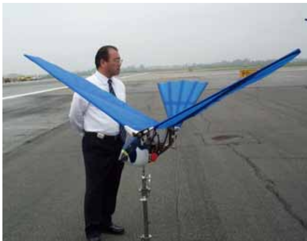
Radio-controlled aircraft, such as this Robo-Falcon™, can be useful as part of an integrated program in dispersing birds from airports and landfills. Considerable training is required to operate these devices in the airport environment (photo by R. A. Dolbeer, USDA).
