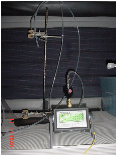
Figure 2-5. Experimental Setup Showing In-Cab Sample Collection
