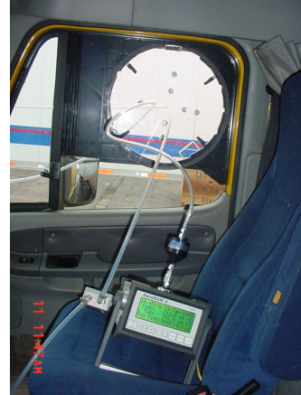
Figure 2-4. Outside Air Sample Probes Connected to DataRAM and Pump for Gas Sample
