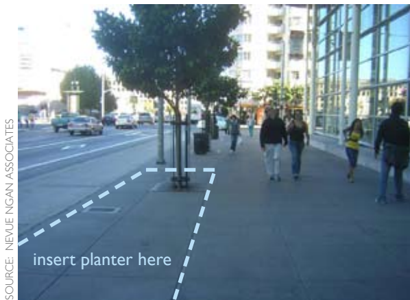
Figure 4-35: Planters can be retrofitted on urban streets with overly wide sidewalk zones. Dashed lines show where a planter could be added.
