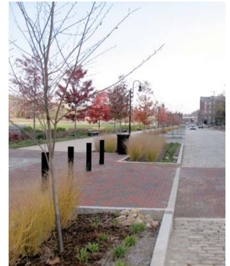
Figure 78: Swale, cobbled street and brick crosswalk.
