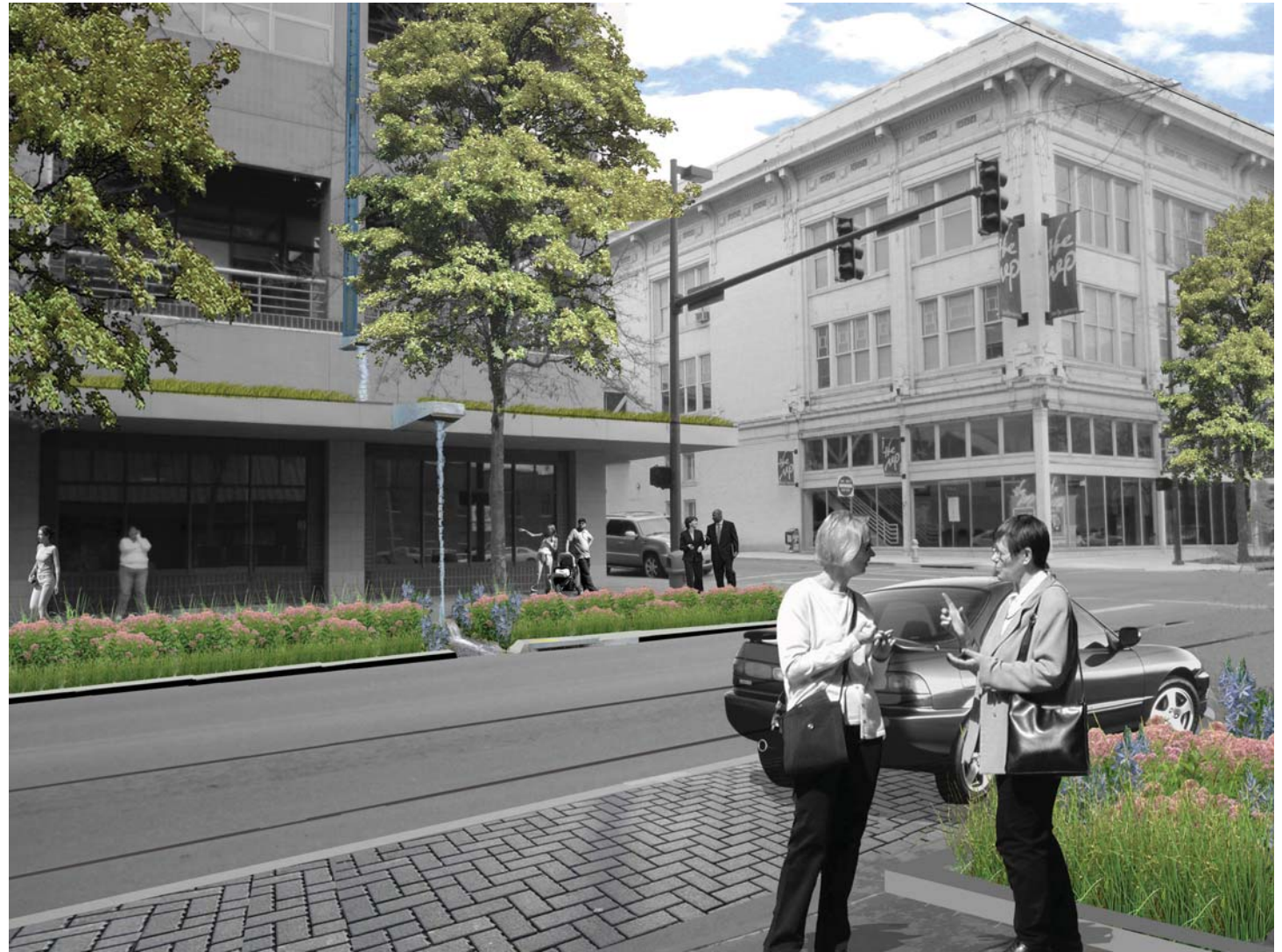
Figure 45: Design concept for a streetscape that includes a streetside rain garden, a parking lane with permeable paving, a downspout rain garden, and a trolley track.
