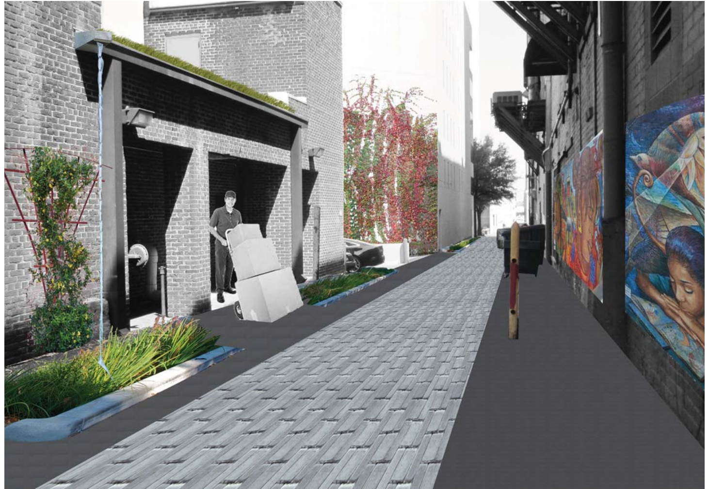
Figure 41: Design concept for a green alley with downspout rain gardens, green roof, permeable pavement, and a mural.
