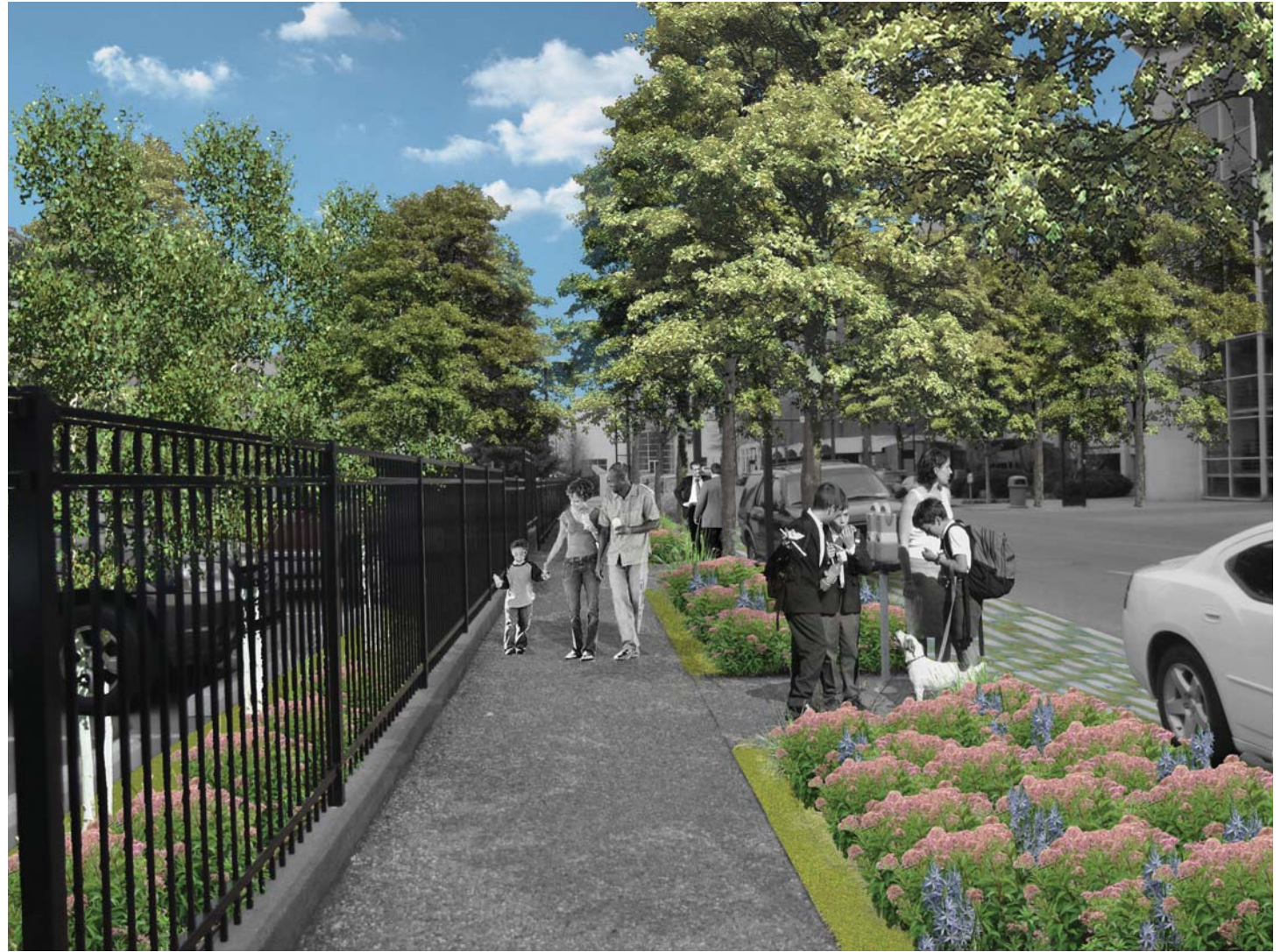
Figure 50: Design concept for a streetscape that includes a streetside rain garden, a parking lane with permeable paving, and a parking lot with a rain garden.
