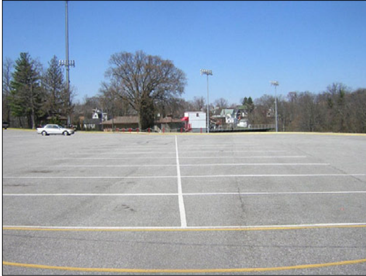
Figure 111. Long parking stalls can be a good opportunity to reclaim a few feet for a stormwater facility.
