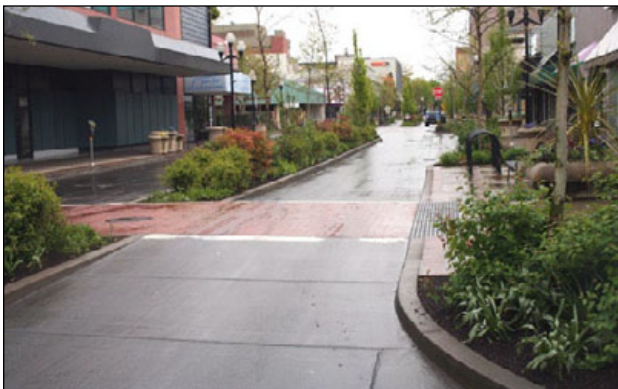
Figure 132. A commercial street with curb extensions and a landscaped median in Eugene, Oregon.
