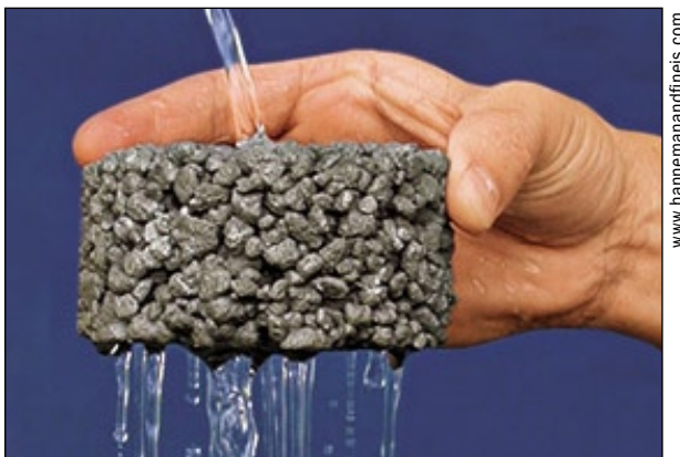
Figure 43. Porous concrete allows water to pass through pore spaces in the aggregate.
