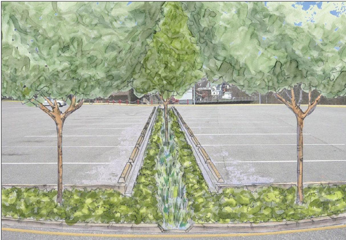
Figure 112. Retrofit potential: 18-foot-long parking stalls are converted to 15 feet, which yields enough space for a 6-foot parking lot swale or planter.
