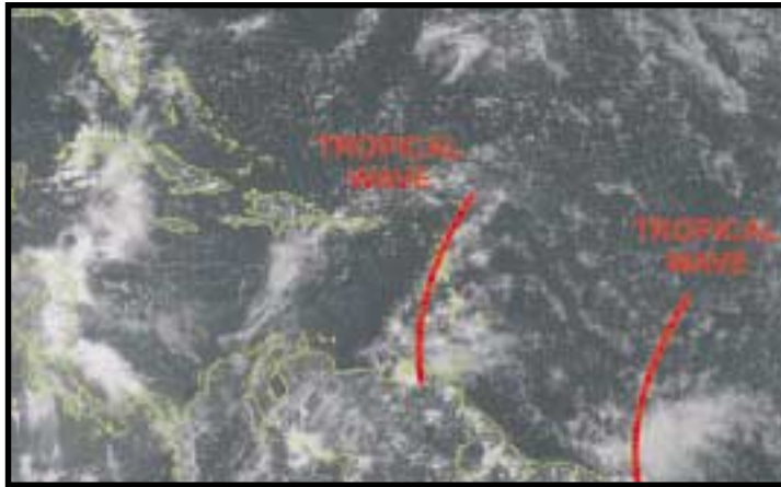
FIGURE 1: GOES-8 image taken at 1415 UTC on 11 June 2000. The axes of two North Atlantic tropical waves are shown in the image. Notice that most of the active weather in the form of showers & thunderstorms, lies east of the wave axis. Wind reports of 20 to 25 KT were recorded in the vicinity of the wave entering the Caribbean Sea near the time of this image.
