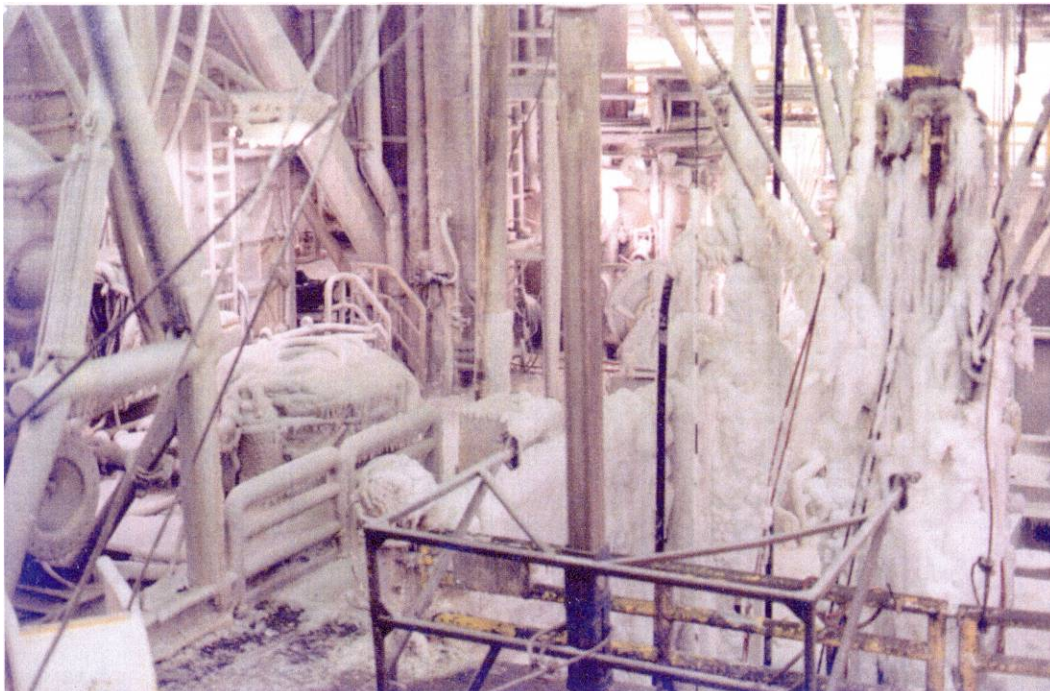
Figure 3. Sea spray icing on the Ocean Bounty in the winter of 1979-1980 in Lower Cook Inlet (photo provided by MMS).
