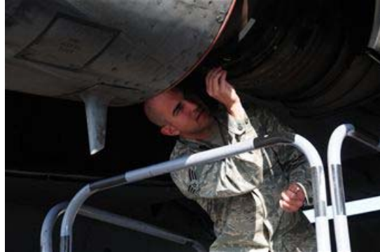
U.S. Air Force Senior Airman Dustin Axtell, 386th Expeditionary Aircraft Maintenance Squadron EC-130 crew chief, checks the tightness of a clamp on an exhaust tail pipe of a C-130 Jan. 22, 2010 at an air base in Southwest Asia. Airman Axtell is deployed from Davis Monthan AFB, Ariz. (U.S. Air Force photo by Staff Sgt. Lakisha A. Croley/Released)
