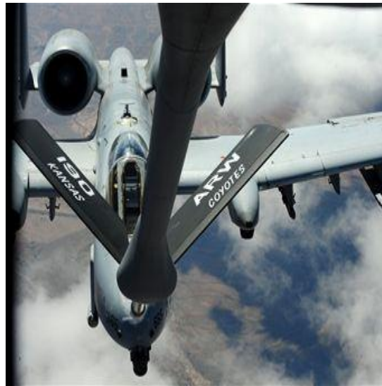
1st Lt. Dan Griffin, a pilot assigned to the 358th Fighter Squadron, readies his A-10C beneath the boom of a KC-135 to receive 2,000 pounds of fuel during an aerial refueling mission in the Tombstone Military Operating Area in Southern Arizona April 27. Lieutenant Griffin is a student in the A-10C Pilot Initial Qualification course and was one of six pilots from his squadron to refuel for the first time. Upon completion of the course in August he will become a fully qualified A-10C attack pilot. (U.S. Air Force photo/Airman Jerilyn Quintanilla)
