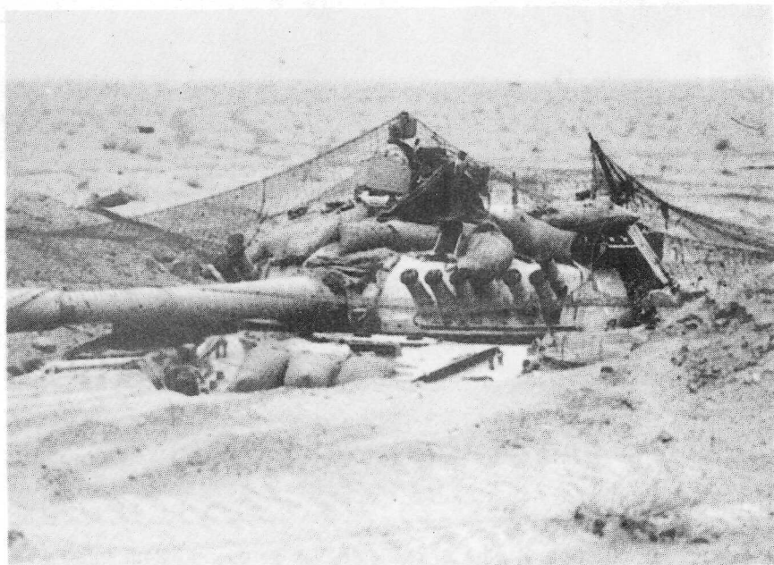
Tawakalna Division T-72 found after the Battle of Wadi al-Batin. The tanks were dug in, exposing only 2-3 feet of turret.
