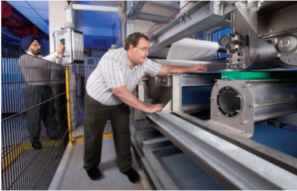
Cotton technologist Paul Sawhney (left) and textile technologist Michael Reynolds prepare an experimental trial for producing a hydroentangled cotton nonwoven fabric on a commercial-grade hydroentanglement system.
