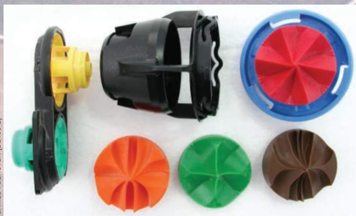
A sprinkler head is easily modified. The body (solid black) can house a single spray plate (orange, green, brown, or red) that alters droplet size and wetted diameter. The body attaches to either side of the dual-nozzle unit (far left): One side applies less water, usually early in the growing season; the other, more water, usually later in the growing season.
