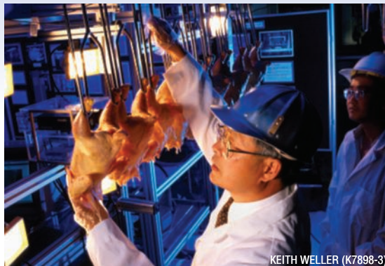
Developed by ARS agricultural engineer Yud-Ren Chen, this automated system could help speed inspection of the billions of U.S. chickens processed annually.
