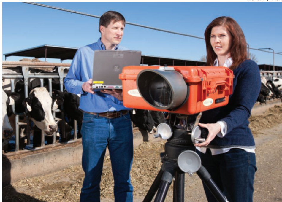
ARS soil scientist April Leytem and research leader David Bjorneberg use open-path ultraviolet-differential optical absorption spectrometry to determine ammonia concentrations at dairy operations in southern Idaho.
