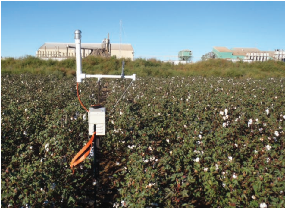
ARS scientists measure the levels of PM2.5 and PM10 in the air outside a cotton gin by surrounding the gin with 126 ambient air samplers, such as this one located in a cotton field near a cotton gin in west Texas.
