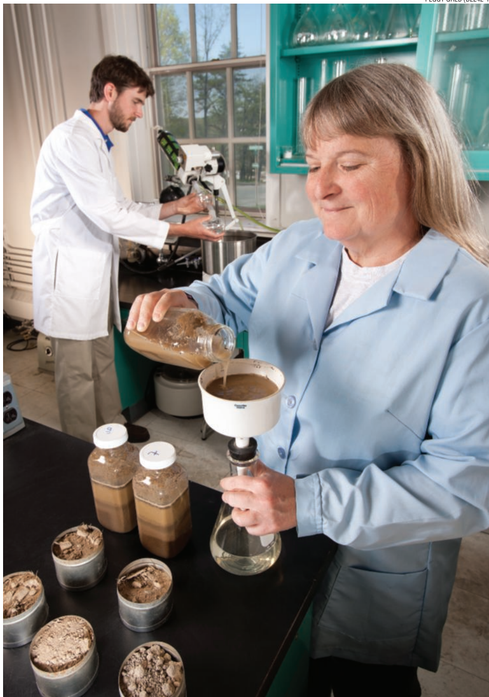
Soil scientist Lynn McKee filters soil samples for pesticide analysis while technician Alex White uses a rotary evaporator to process pesticide samples.
