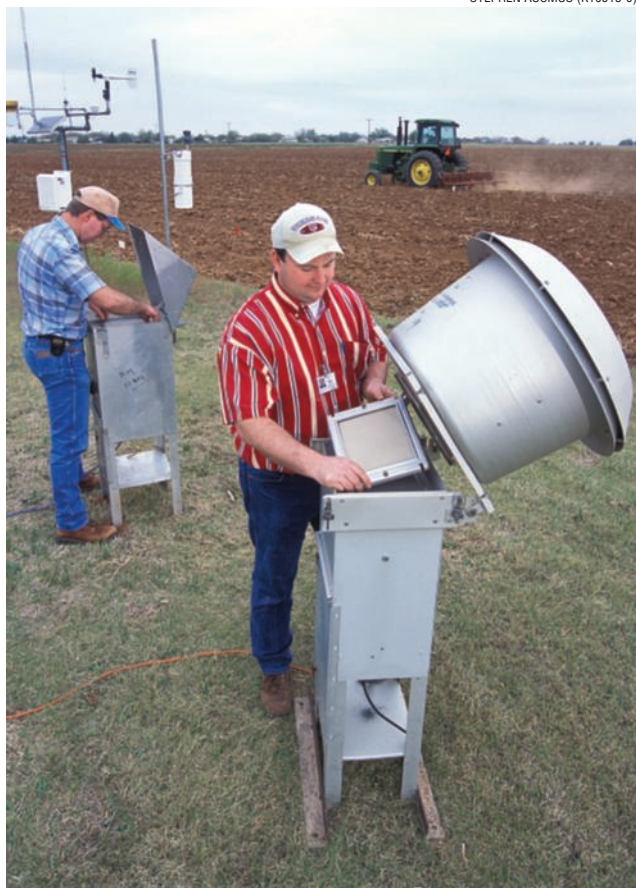
An ambient PM10 high-volume sampler in a west Texas dust storm. A storm like this exposes samplers to dust particles greater than 10 micrometers, and larger dust particles increase the overall error associated with ambient air samples.
