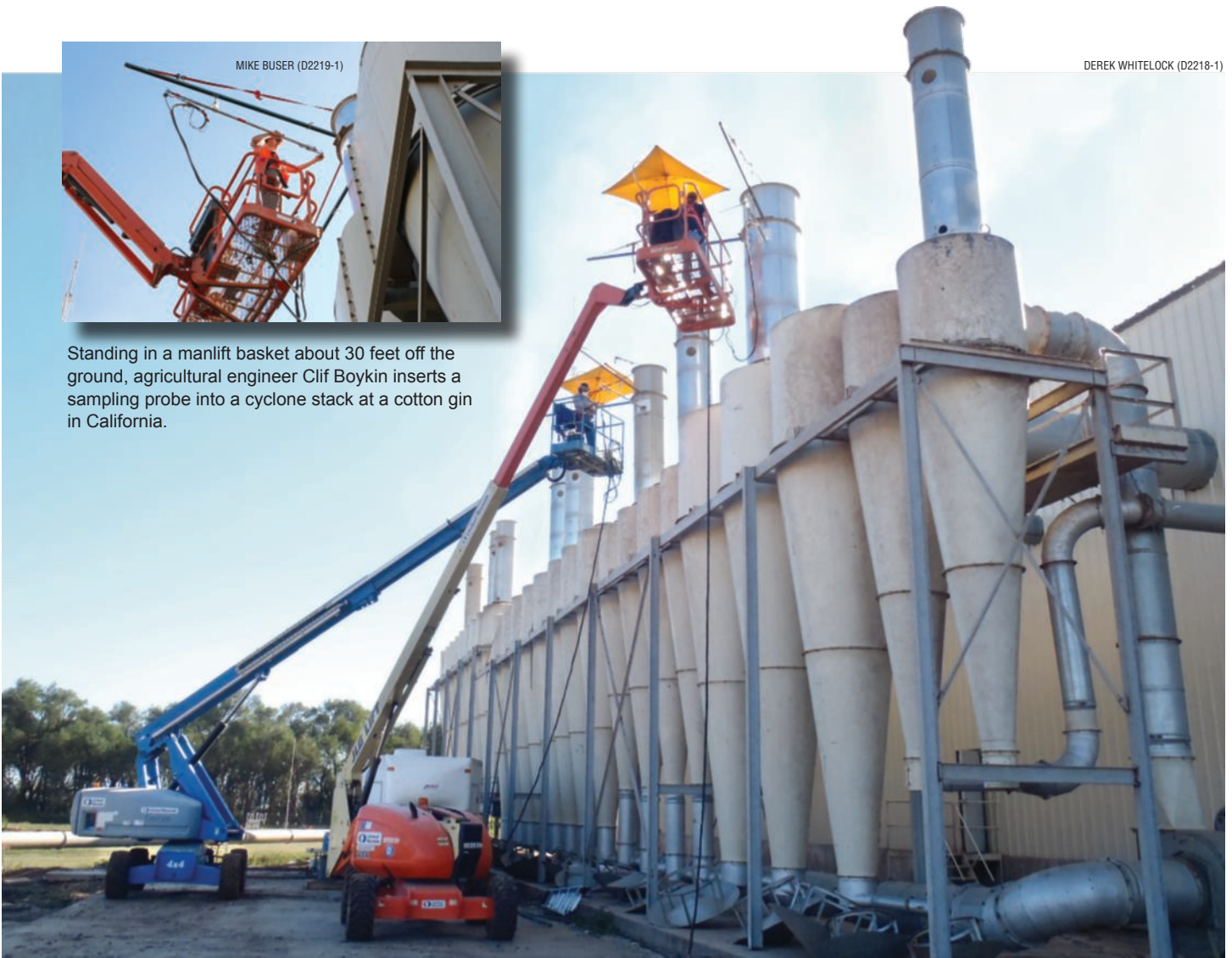
To accurately determine the total PM 10 and PM 2.5 emissions from a cotton gin in west Texas, ARS biological science aids Arnold Gomez and Bud Welch directly sample exhaust from the gin's many cyclones. Samples are then brought back for processing in the ARS Air Quality Laboratory in Lubbock.
