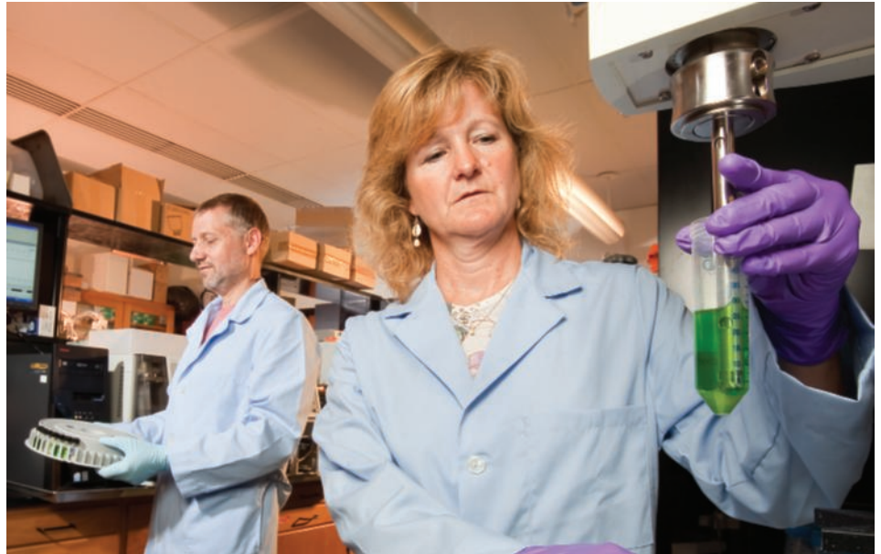
At the ARS Natural Products Utilization Research Unit in Oxford, Mississippi, support scientist Susan Watson extracts a sample of pigments from leaf tissue for high-performance liquid chromatography analysis by plant physiologist Franck Dayan.
