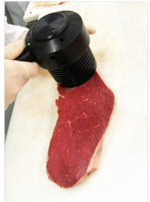
A visible and near-infrared reflectance (Vis/NIR) spectroscopy probe head is applied to a top sirloin steak to predict tenderness and color stability.
