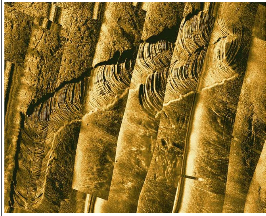
FIGURE 2.2 Dredging scars from a CSD operation in Red Brook Harbor, MA.
