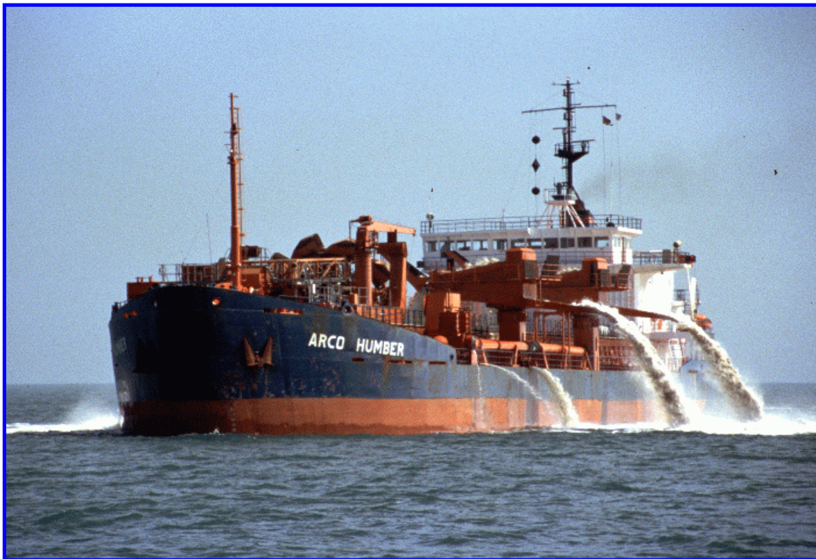
Plate 1. Typical marine aggregate dredger loading a cargo and discharging screened material from reject chutes. Overspill losses from the cargo hold can also be seen. Copyright ©MESL-PhotoLibrary.
