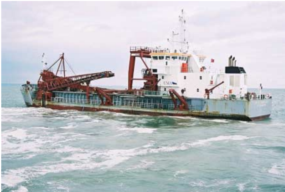
Plate 1.5a. City of Chichester 2300 tonne capacity dredger operated by UMA working on the North Nab licence.
