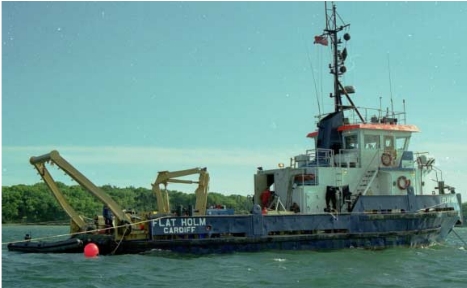
Plate 1.4. 24m Research and survey vessel M.V. Flat Holm used for the surveys at Licence Area 122/3
