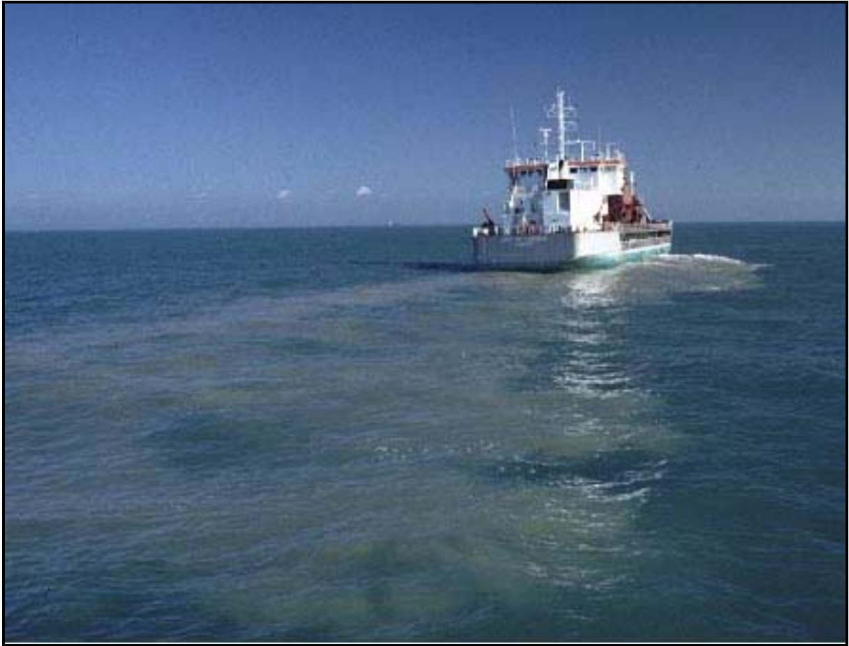
Plate 6.4. Photograph showing the plume of dispersing outwash being carried westwards on the ebbing tide during loading of a cargo at station 126 of the North Nab Study site by the City of Cardiff on 13.03.99.
