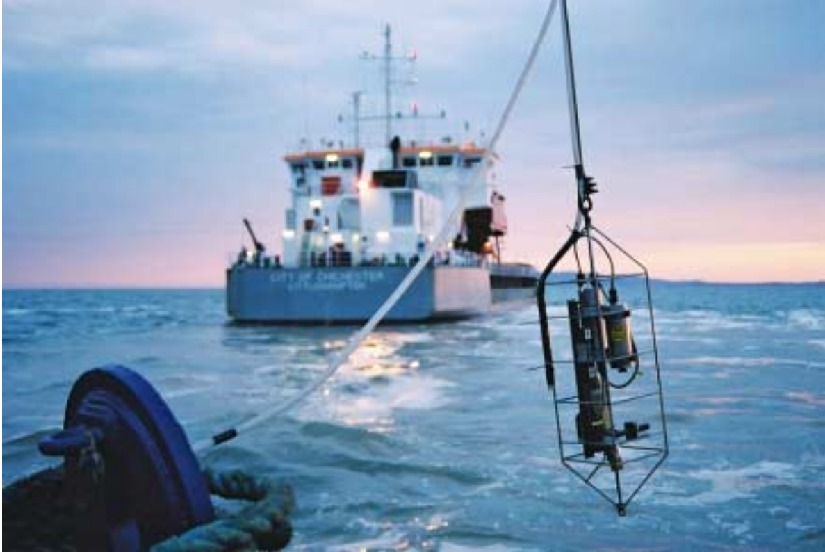
Plate 4.3a. Deployment of water sampling equipment in the plume generated by the City of Chichester
