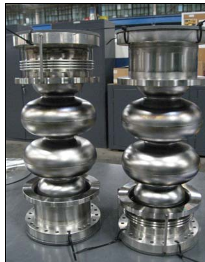
Figure 3. Two finished NSLS-3HC SRF cavities.
