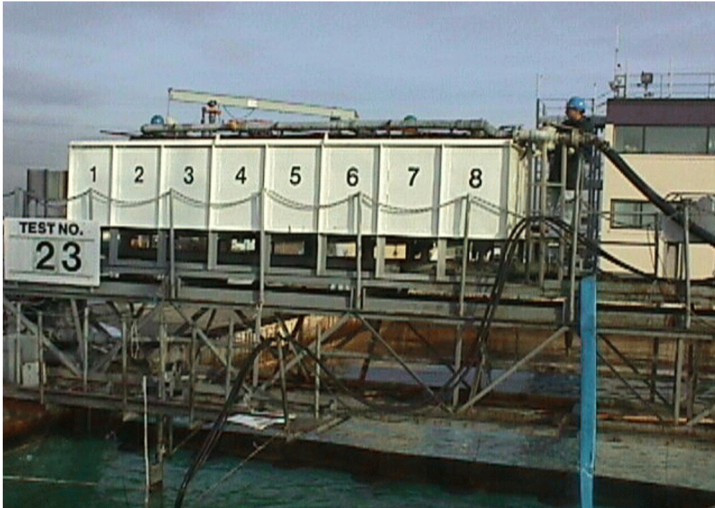
Figure 3. Recovery tank on auxiliary bridge.
