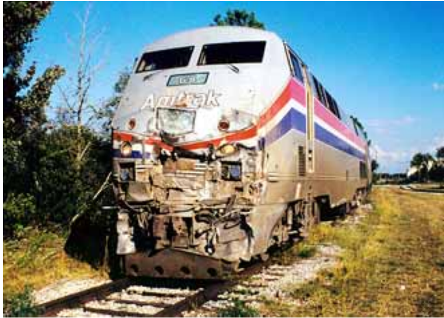
Figure 8. Amtrak locomotive after collision.
