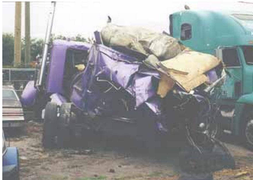
Figure 8a. Rear view of pusher tractor after collision.
