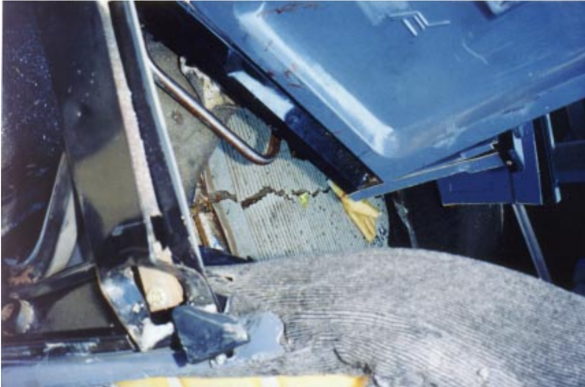
Figure 7. Cracked plywood flooring in Lenoir City specialty bus
