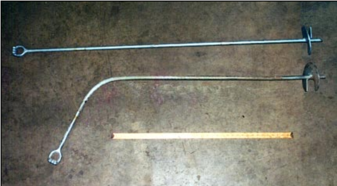
Figure 2. Unused anchor (top) and accident anchor after removal from accident site
