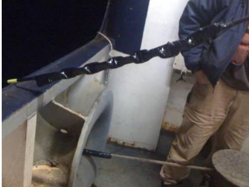
Figure D.19: One of the four lengths of chain used to weigh down the cable.
