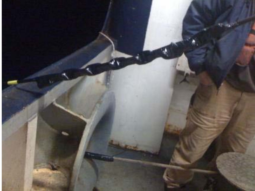
Figure 6. One of the three lengths of chain used to weigh down the cable.
