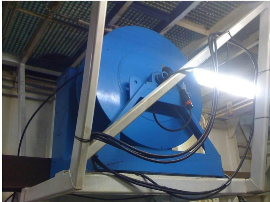
Figure D.19: Hydrophone cable on winch
