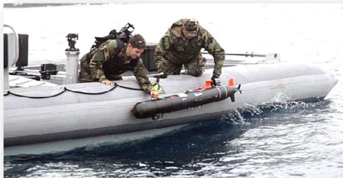
Navy Explosive Ordnance personnel deploying an unmanned underwater vehicle (UUV) from an 11-m jet-water propulsion Rigid Hull Inflatable Boat (RHIB)
