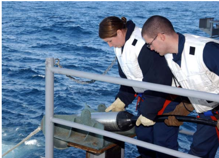
Figure 1. NIXIE torpedo countermeasure source (tow body) being deployed from the back of a U.S. Navy ship.
