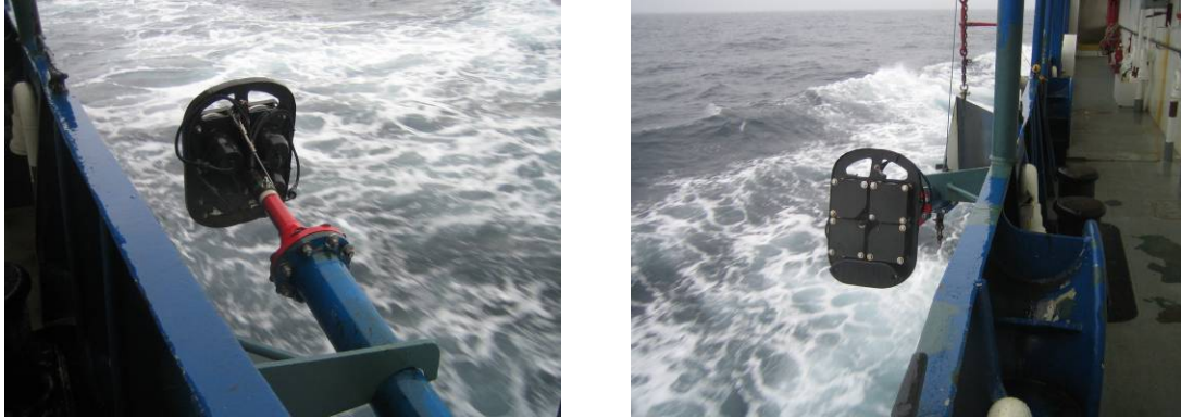
Figure 5. The Geopulse 3.5 kHz sub-bottom profiler mounted on a swinging pole on the port side of the R/V Mt Mitchell .
