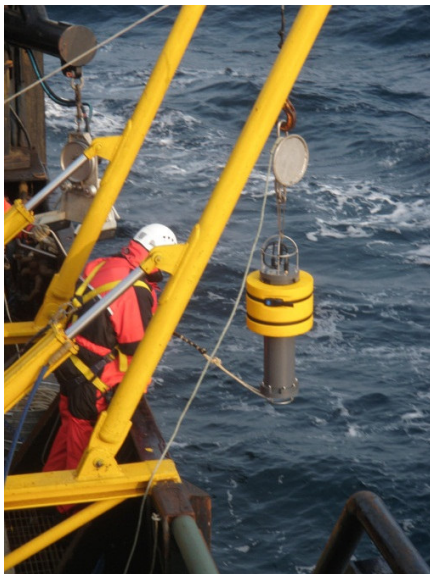
FIGURE 3. AMAR autonomous acoustic recorder for acoustic monitoring of drilling activities.
