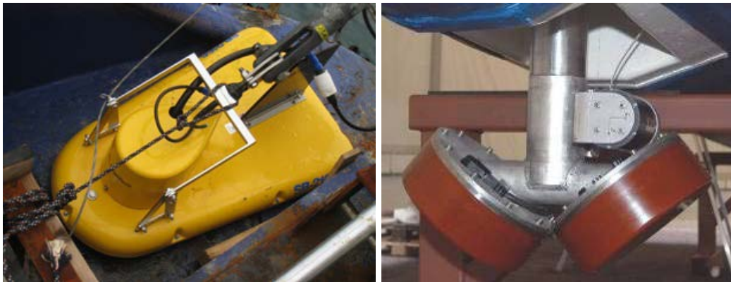
FIGURE 3.4. EdgeTech 3100 SB-216S sub-bottom profiler towfish (left) and Kongsberg EM 3002 multibeam sonar (right, photo source: http://www.gserentals.co.uk ).
