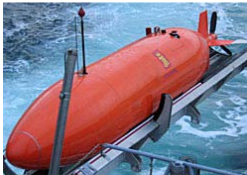
FIGURE 3.5. Kongsberg HUGIN 1000 autonomous underwater vehicle (AUV) with onboard sub-bottom profiler, multibeam sonar and side-scan sonar (photo source: http://www.km.kongsberg.com ).
